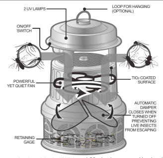
Flying insects are attracted to the unit by the UV light and  $CO_2$  that is generated by the photo-catalysis between the UV lamps and the special  $TiO_2$  coating. The fan then pulls the insects into the screened base, trapping them until they dehydrate and die. The base can be removed, allowing the contents to be periodically emptied into the trash. The see-through screen shows the insects trapped in the compartment, alerting you when the cage needs to be emptied.
